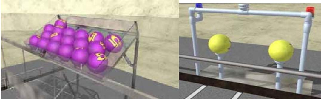
The Ball Release stores eighteen (18) Small Balls and is mounted above each Alliance Station.
